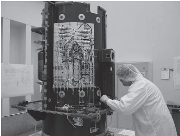
Working in a clean room facility at JPL, a mission engineer assembles the xenon feed system of Dawn's ion propulsion system.
